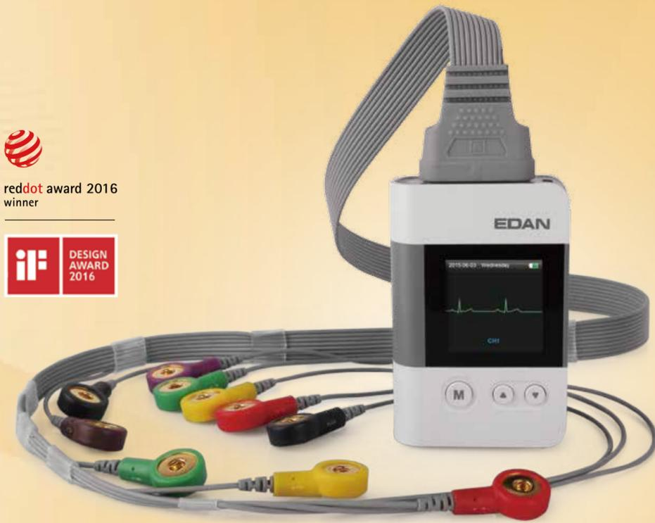
EDAN Holter Recorder is designed with low power consumption, which enables it to record as long as 8 days with a single piece of Li-ion battery.
